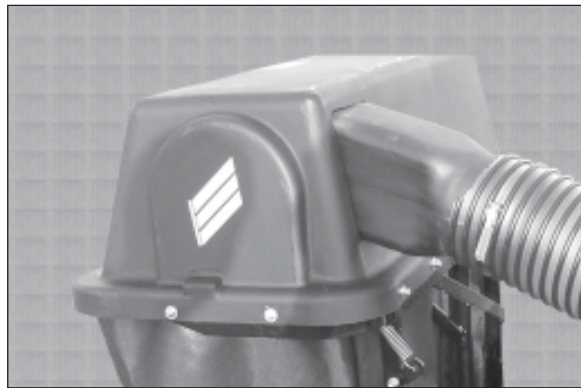
Figure 17 Install the grass tube and secure into place using two hose clamps found in the hood assembly box.
