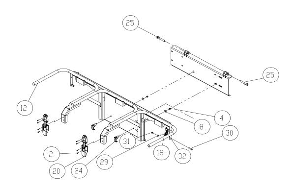
BOLT THE 3-BAG FRAME TO THE BACKPLATE MOUNT USING THE DECK HEIGHT PINS (#25) AND SWELL LATCHES (#24).
