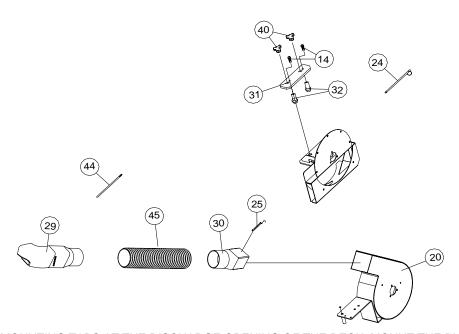
USING THE MOUNTING TABS AT THE DISCHARGE OPENING OF THE DECK, MOUNT THE BLOWER ASSY TO THE DECK BY SLIPPING THE MOUNTING TABS INTO THE SLOTS FOUND ON BLOWER MNT WLDMT. SECURE IN PLACE USING RING PIN (#24). TIGHTEN DOWN KNOBS (#40) UNTIL ADAPTER RAMS (#32) ARE TIGHT AGAINST THE DECK. FASTEN THE GRASS TUBE (#45) TO THE HOSE ADAPTERS (#29 & #30) USING GRASS TUBE CLAMPS (#44). ATTACH BLOWER TIE DOWN (#25) TO BLOWER HOSE ADAPTER (#30) USING HARDWARE FROM BOLT BAG.
