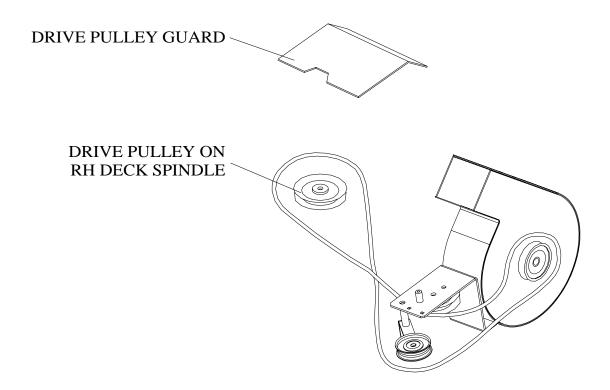
Route the blower drive belt so that the "V" side of the belt rides in the "V" groove of the drive pulley mounted on the RH blade spindle, the driven pulley mounted on the outside of the blower, and the stationary idler pulley bolted to the blower. The "flat" side of the drive belt should ride against the flat groove found on the spring tensioner pulley. Refer to diagram above for illustration of belt routing.
