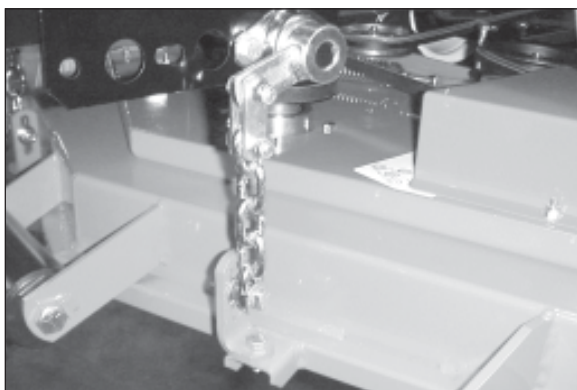
Figure 7 Remove the left front deck lift chain assembly and L-bracket by loosening the 3/8" whizlock nut and bolt from the deck mount tab and loosening the 3/8" nyloc nut and bolt that secures the chain assembly to the deck lift crank.
