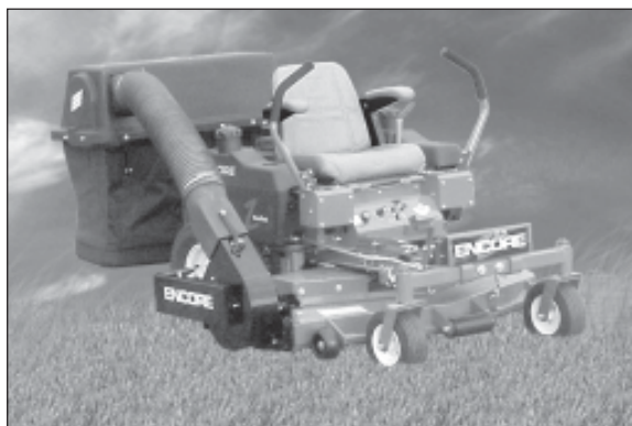
Figure 19 This completes the installation of your new Encore grass catcher system. Note: When engaging the PTO switch; always make certain the unit is running 3/4 to full throttle so as to prevent stalling.
