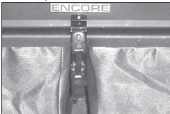
Figure 14 Close the grass catcher hood & secure the hood latch.
