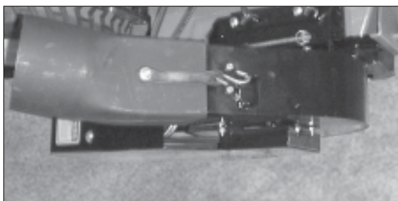
Figure 16 Fasten the tie-down strap to the blower hose adapter.
