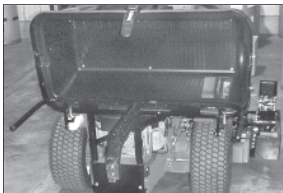
Figure 12 Slide the assembled hood and frame onto the rear skid bars. Let the assembly slide all the way down to the grass catcher brace.
