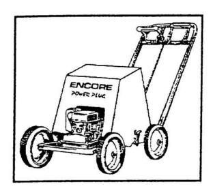
Handle: Slide the handle onto the frame pegs. The control levers should be facing up. Insert The (2) 1/4" bolts and fasten with the (2) 1/4" Locknuts or the hardware that is provided.
