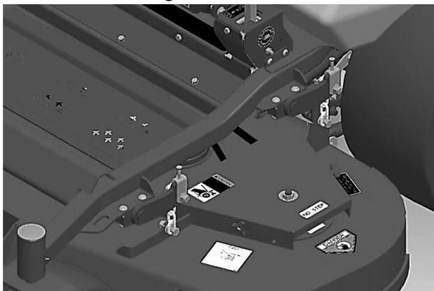
11. If the four deck links do not have enough adjustment to achieve accurate cut height with the desired rake, the single point adjustment can be utilized to gain more adjustment
