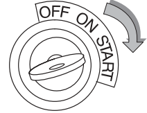
Typical starter switch
