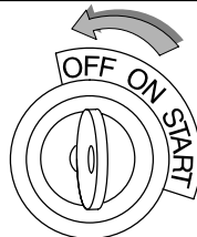
Typical starter switch
